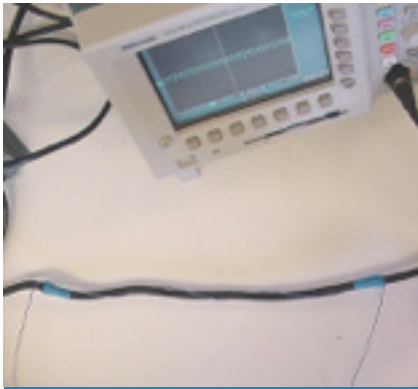
BLUE TEST WIRE AROUND MOTOR CABLE
